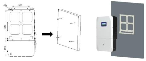
**Step 2**: Attach the Hanging rack to the wall using 4 expansion screws. Lift the inverter, place the inverter on the Hanging rack, and tighten the screws on both sides of the lower part.
