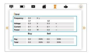
① Display the working parameters on the grid, including **Frequency**,
