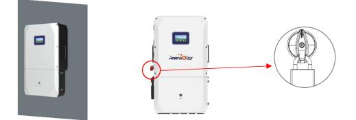
**Step 4**: The two latches on the lower right of the inverter open upward to open the waterproof cover. If you need to remove the display panel on the top half of the machine, use a hexagonal screwdriver to remove the six screws on the top. Wiring box conduit plugs, Conduit plugs are provided for linch conduit fittings. If used conduit fitting is not 1 inch, an appropriate conduit adaptor should be used.
