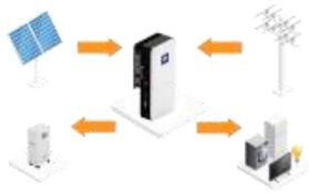
B.On charge time, solar energy will charge battery as first priority.then the excess solar energy will supply power to loads.If solar energy is not sufficient to charge battery and supply loads,grid will supply all the connected loads with solar energy together.
