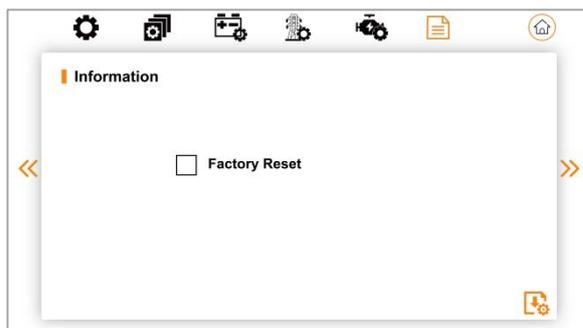
This interface is used to reset the inverter.
