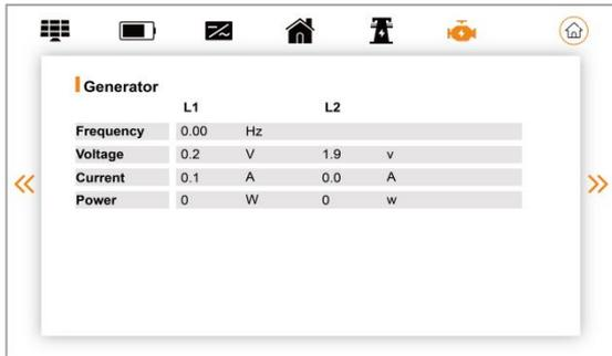
Display the working parameters of the generator, including **real-time voltage, current, and power.**
