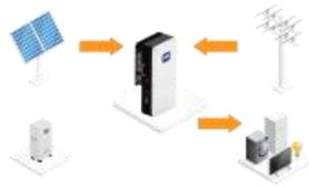
B.Solar energy provides power to the loads as first priority,if solar energy is not sufficient to power all connected loads, Grid energy will supply power to the loads at the same time.
