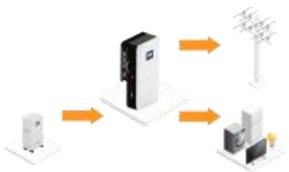
B.On discharge time,if load power is less than battery power,battery will supply power to loads as first priority,the excess power will be feed to grid.
