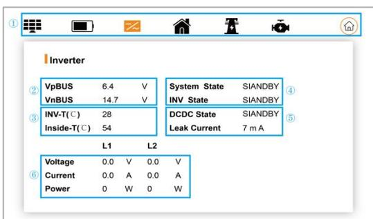
①Users can click on the icon above to switch device status data (PV, Battery, Energy Storage Inverter, Load, Grid, BUS) and return to the Home Page. (not to be repeated later)
