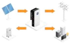
A.On charge time, solar energy will charge battery as first priority.The excess energy will supply power to the loads.If solar energy is sufficient to supply loads and charge battery,and If there's still some extra energy,then the excess power will feed the power to grid.
