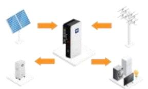
B. Solar energy will charge battery as first priority, if solar energy is excess, the excess power will supply load. If solar energy is not sufficient to charge battery and supply loads, grid will supply power to loads.
