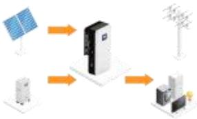
B.Solar energy provides power to the loads as first priority ,if solar energy is not sufficient to power all connected loads, battery energy will supply power to the loads at the same time
