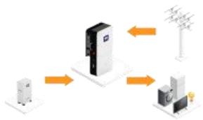
C.On discharge time,if load power is more than battery power,battery and grid will supply power to the loads at the same time.
