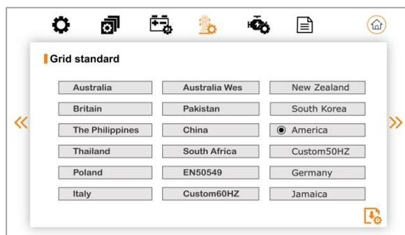
This interface is used to select Grid standard. Users can set and switch grid standards according to their needs.
