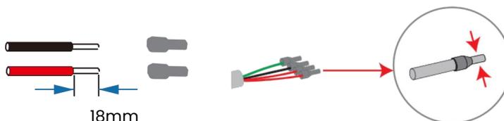
**Step2.** Connect the cables to the BACK-UP: Load port of the inverter.
