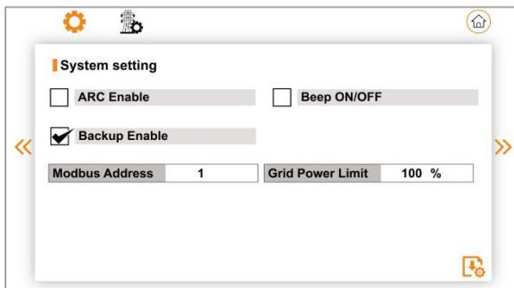
**ARC Enable:** ARC detection function.
