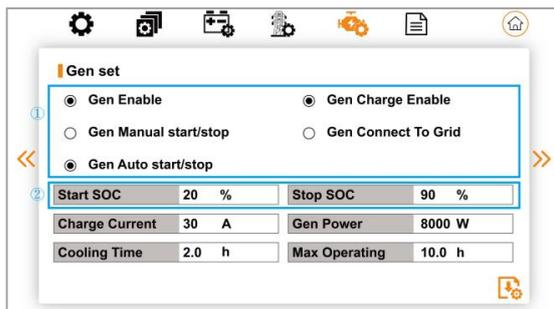
As shown in the picture on the left, select Gen Enable, Gen auto and Gen charge enable. Set generator on, off SOC or voltage, charging current, generator power, stop cooling time, maximum running time.
