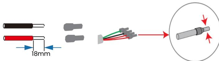
**Step4.** Cross the Grid cables through the grid port, Connect Grid cables to Grid terminals.
