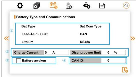
① Set Battery Type and Battery Communication method.
