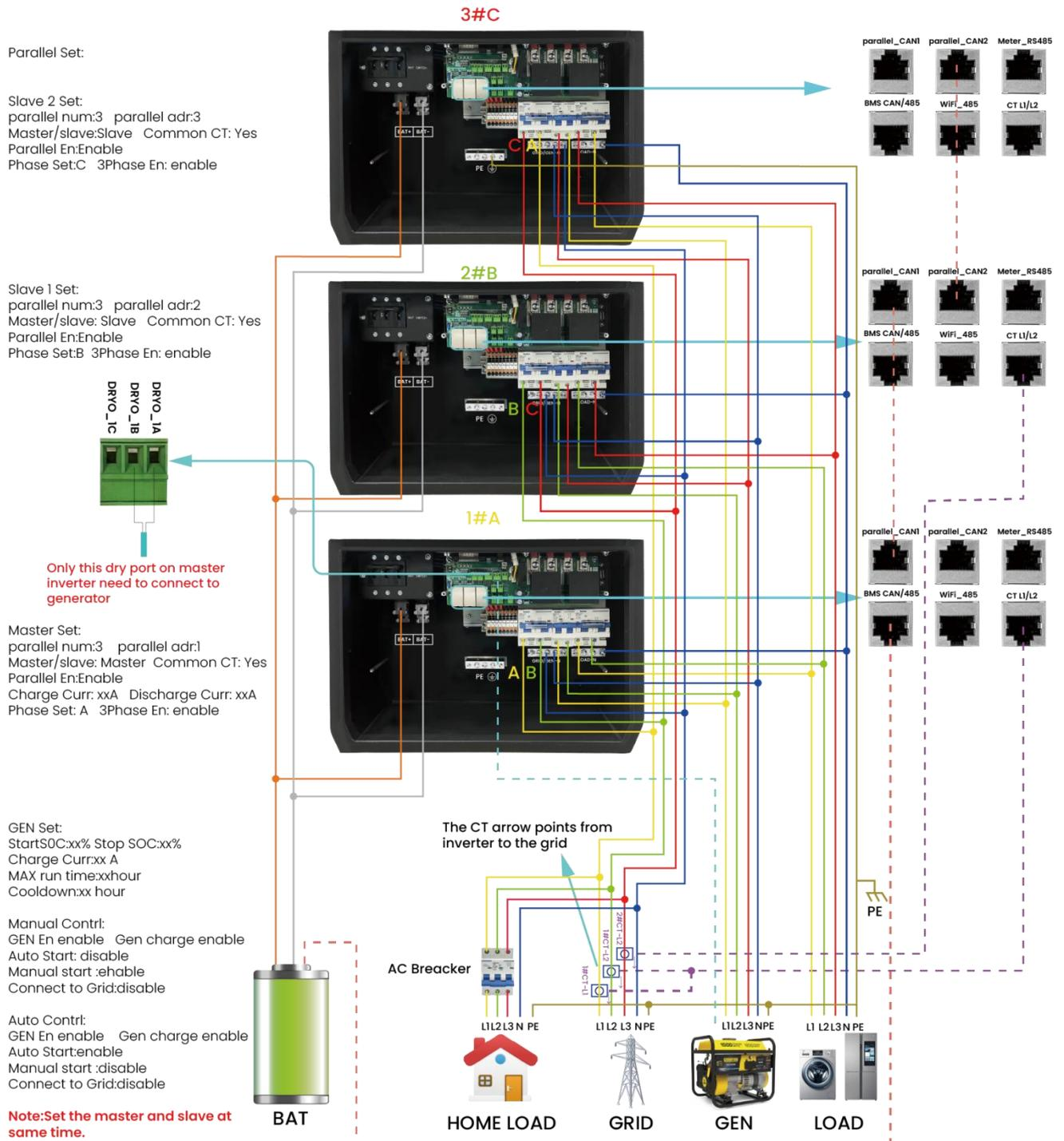
Multiple inverters can be installed together to deliver more power. When AC loads are present, all units effectively share the load. The system diagram is as follows.
