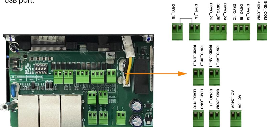
**DRY1\_1B/DRY1\_1:** Used to start the Inverter driver.
