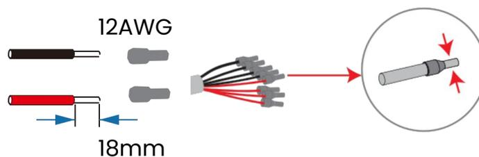
**Step2.** Cross the PV cables through the PV port, Connect PV cables to PV terminals.
