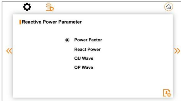
**Power Factor:** The input value should range between L0.80 and L0.99 or C0.8 and C1.00.
