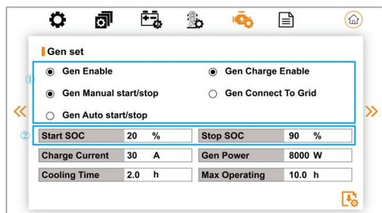
As shown in the picture on the left, select Gen Enable, Gen Manual and Gen charge enable. charging current, generator power, stop cooling time, maximum running time.
