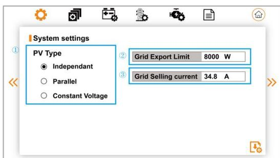
① Users can set PV types, including Independent, Parallel and Constant Voltage.
