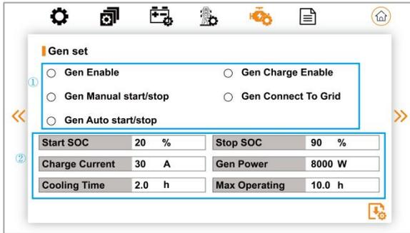
① Diesel generator enable settings:
