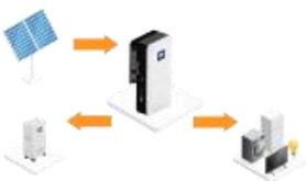
B.Solar energy provides power to the loads as first priority ,if solar energy is not sufficient to power all connected loads,battery energy and solar energy will supply power to the loads at the same time.
