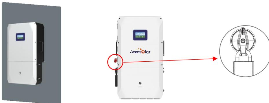
**Step 4:** The two latches on the lower right of the inverter open upward to open the waterproof cover. If you need to remove the display panel on the top half of the machine, use a hexagonal screwdriver to remove the six screws on the top. Wiring box conduit plugs, Conduit plugs are provided for 1inch conduit fittings. If used conduit fitting is not 1 inch, an appropriate conduit adaptor should be used.
