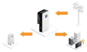
A.On charge time,grid will charge battery and supply power to the connected loads at the same time.
