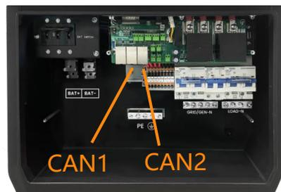
For parallel communication, CAT 5 cables are needed. The units should be connected hand by hand.
