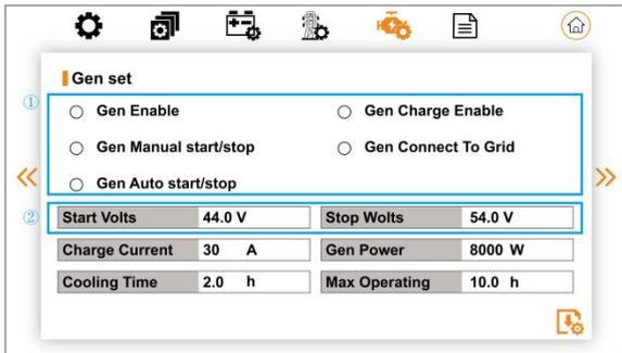
**Start Volt:** Generator in automatic mode. When the volt of battery is lower than the setpoint, the Generator dry
