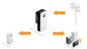
2. When Grid, Battery is available (PV is disconnected): Grid will supply power to load and charge battery at the same
