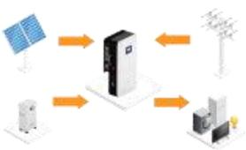
C.Solar energy provides power to the loads as first priority, if solar energy and battery are not sufficient to power all connected loads, utility energy(Main Grid)will supply power to the loads with solar energy at the same time.
