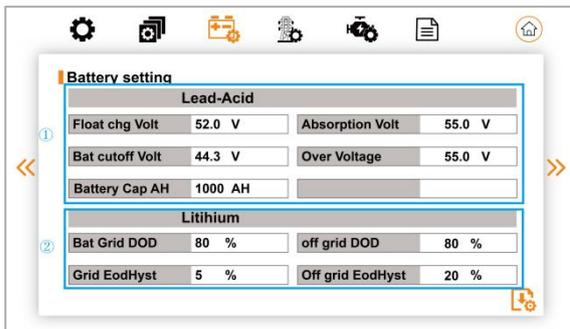
① Settings required when using lead-acid batteries
