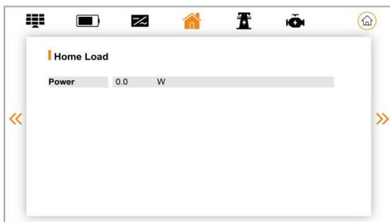
When set Home load EN to "ENABLE", if you have a load connected to the mains port, you can see its Home load power.
