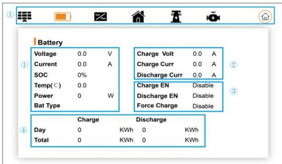
① Display the working parameters of the battery, including **real-time voltage, real-time current, battery surplus capacity, battery temperature, battery power, and battery type.**
