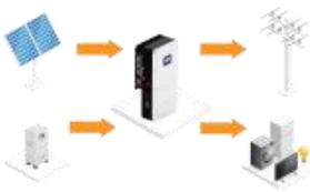
C.On discharge time, solar energy provides power to the loads as first priority, if solar energy is sufficient to supply loads,and if there's still some extra energy from solar energy ,then the excess power and battery will deliver the power to the grid at the same time.
