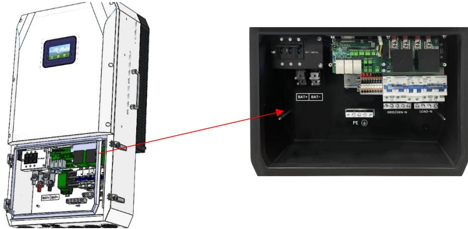
**Step 5:** Pass the corresponding conduit and fasten the joint.
