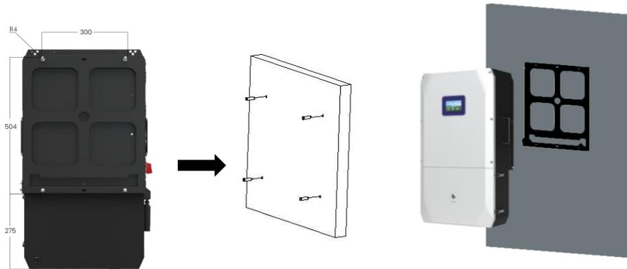
**Step 2:** Attach the Hanging rack to the wall using 4 expansion screws. Lift the inverter, place the inverter on the Hanging rack, and tighten the screws on both sides of the lower part.
